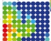
Group array analysis of an inhomogeneous distribution of Cu-nanoparticles on a graphite substrate. Colour scale used to represent relative elemental concentration.
