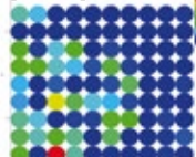
Group array analysis of an inhomogeneous distribution of Cu-nanoparticles on a graphite substrate. Colour scale used to represent relative elemental concentration.
