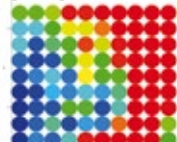
Group array analysis of an inhomogeneous distribution of Cu-nanoparticles on a graphite substrate. Colour scale used to represent relative elemental concentration.
