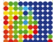
Group array analysis of an inhomogeneous distribution of Cu-nanoparticles on a graphite substrate. Colour scale used to represent relative elemental concentration.
