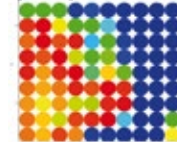
Group array analysis of an inhomogeneous distribution of Cu-nanoparticles on a graphite substrate. Colour scale used to represent relative elemental concentration.
