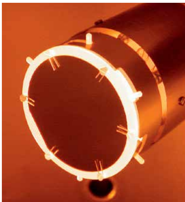
Heated molyblock with Silicon wafer
