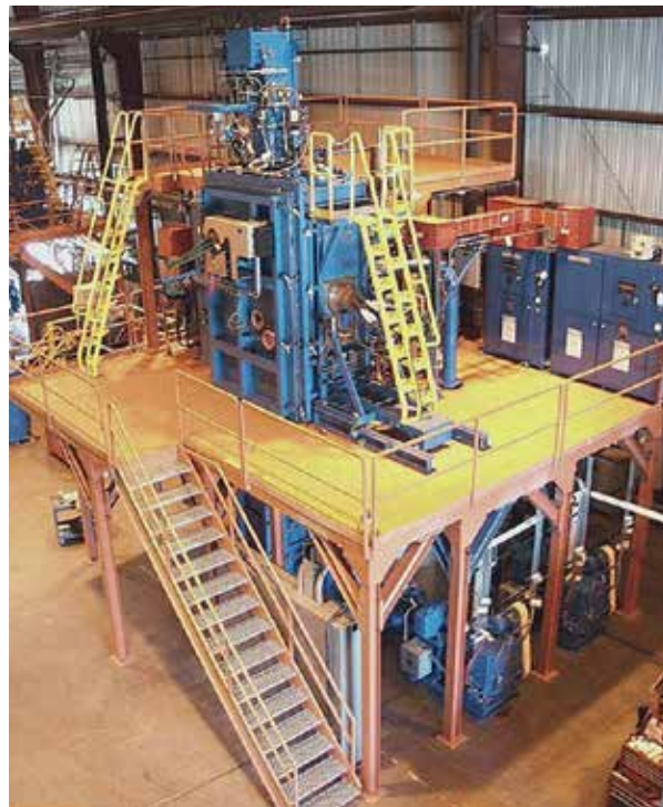
Vacuum furnace for metal powder production
